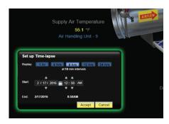
Review floor plans, equipment graphics, trending and alarms over a past period of time so you can quickly identify and resolve building control issues.
